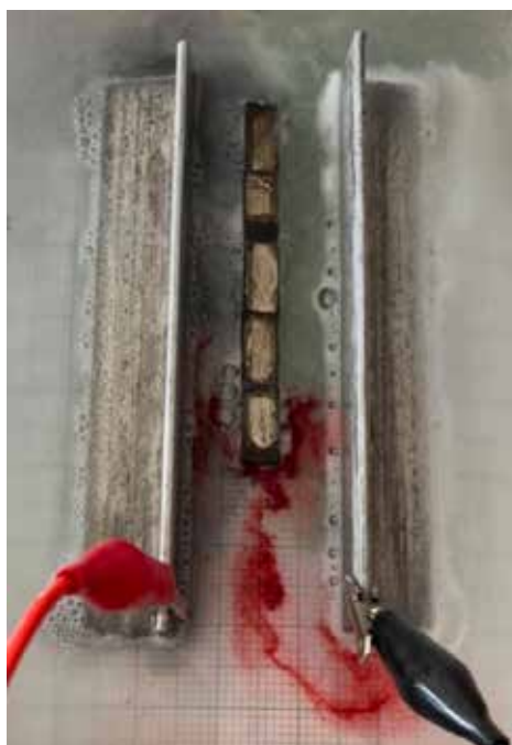
Figure 7: 8042 - Erratic movement with salt sedimentation.
