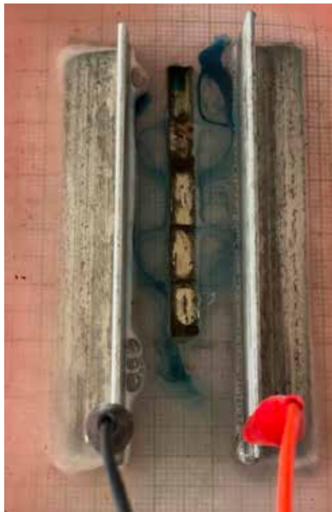
Figure 6: MHD flow after change in electrical polarity
