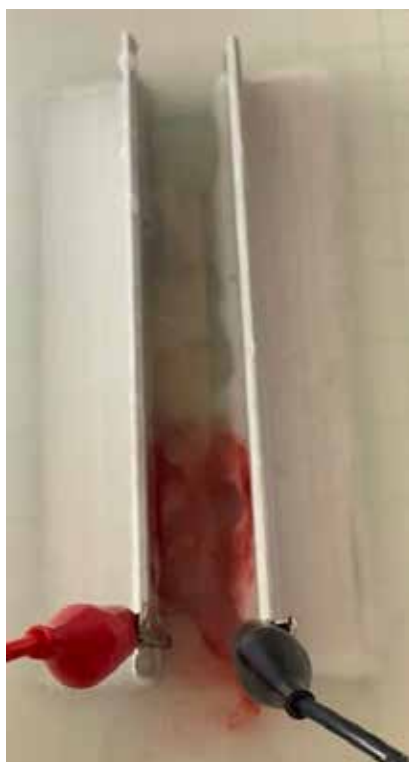
Figure 8: 8054 - Erratic movement when electrode distance is quite small.
