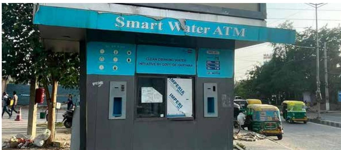
Water ATMs (Anytime Water Machines) are water dispensation systems that can be operated automatically with a coin or smart card, or manually. These are operated by private companies and are a good augmentation to distributing safe drinking water in localities. Most of these ATMs leverage the RO (reverse osmosis) method of filtration. They are often installed at public places like railway stations, bus stops, crowded shopping areas where the need for potable drinking water is acute.
